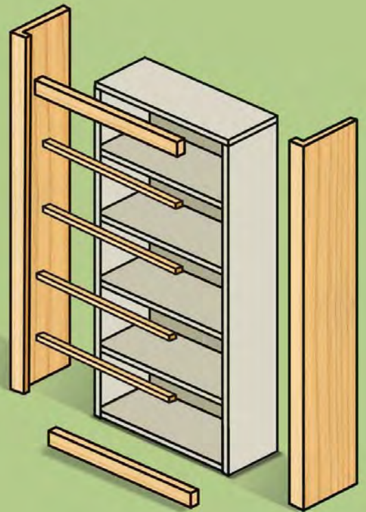
The secret to Wood-Tek's superior strength is its unique design, a rigid four-post steel frame clad in rich wood.
